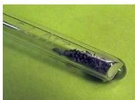
*Before any heating, glass ampules can be conveniently engraved using a diamond-coated engraving tool. During heating at 500 °C for 30 minutes, Indiana Zinc reacts quantitatively with water. The zinc surface becomes oxidized and turns gray and dull.*
