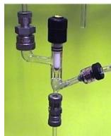
*The vacuum line connects via Ultra-Torr® fitting to the top left. From the right side, the syringe pierces through a septum (see also picture below). Another Ultra-Torr® connection at the bottom holds the 6mm o.d. glass ampule containing zinc. This setup is specialized for the injection of liquid water with a syringe. Other arrangements are necessary if water is derived from fluid inclusions or from combusted organic matter.*
